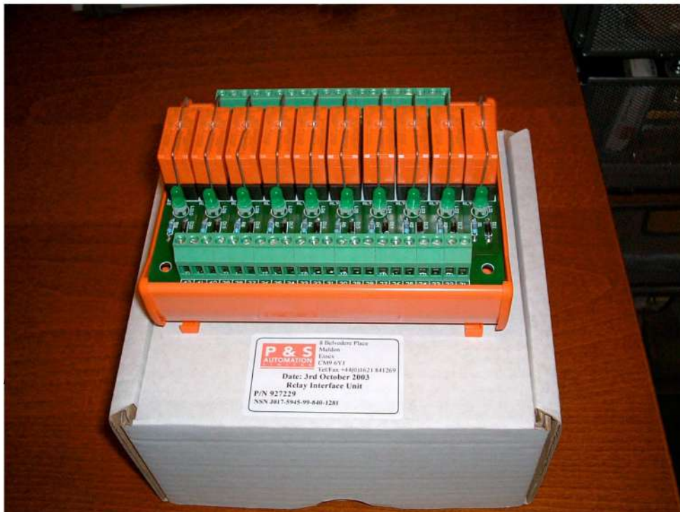
Relay Interface Module Unit
